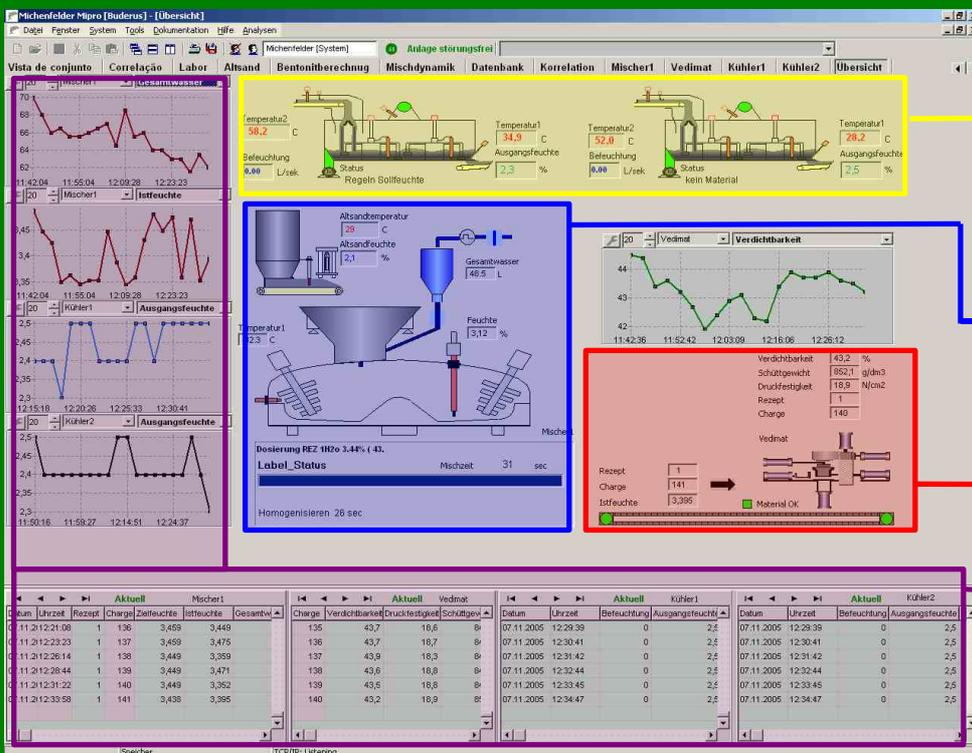
Two mixer coolers, each with two moisture electrodes and two temperature probes, indicating real-time values
